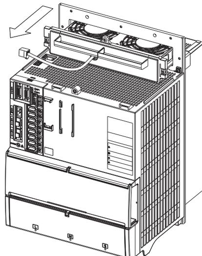
(4) When installing the fan unit, insert the sheet metal of the fan unit into the fin rails.
