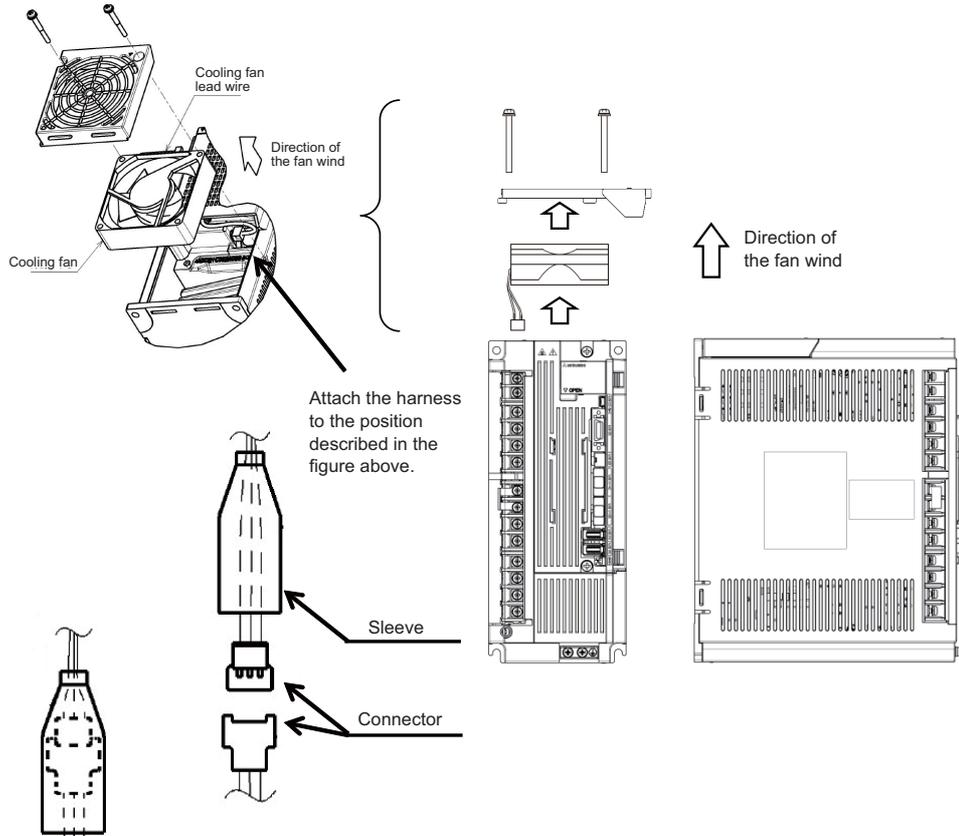
Insert the connector so that it will reach the end of the stopper when assembling.
