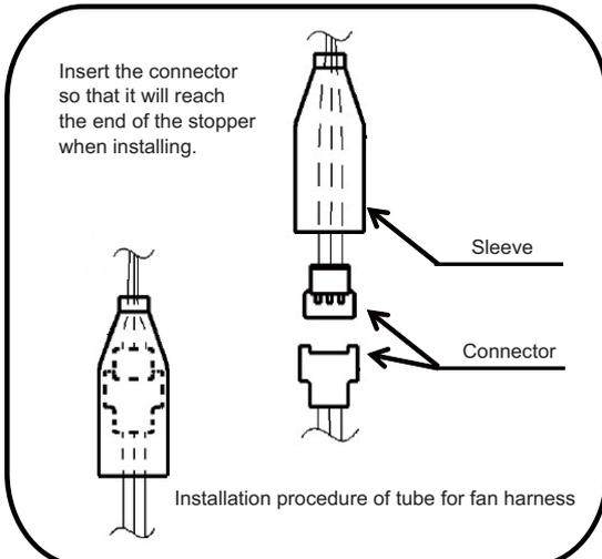
Place the fan harness inside the chassis using the positioning boss for the chassis. Fold the harness to put it inside so that it will not be stuck by the cooling fan.
