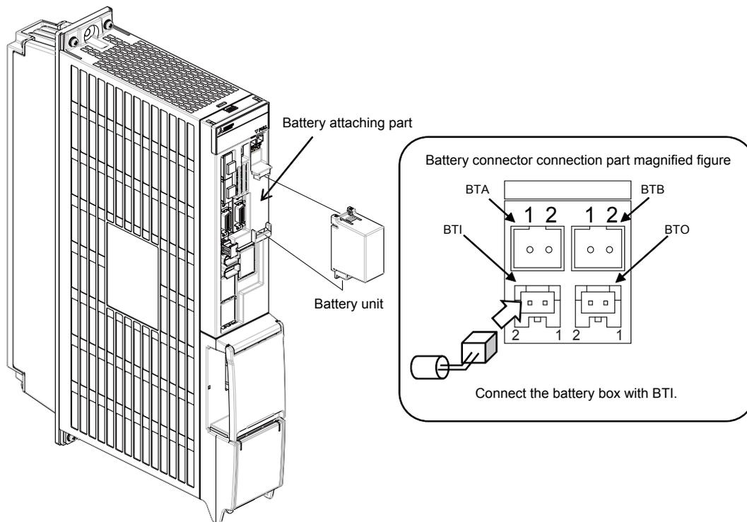
**<Replacement procedure for the battery unit MDSBTBOX-LR2060>****Possible backup period**
