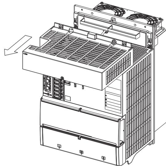
(3) Remove the fixing screws from the fan unit. Disconnect the connector on the top and pull out the fan unit.
