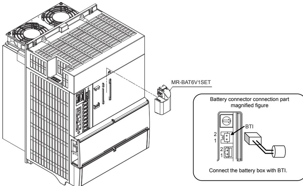
**<Replacement procedure for the battery unit MDSBTBOX-LR2060>****Possible backup period**
