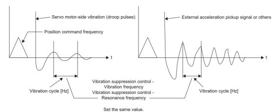
**3.** Set "Vibration suppression control - Vibration frequency damping setting" and "Vibration suppression control - Resonance frequency damping setting".
