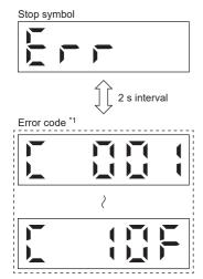
If an error occurs during the one-touch tuning, the tuning will be forcibly terminated and the stop symbol and error code (C 001 to C 10F) will be displayed by turns with 2 s interval.
