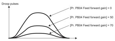
When [Pr. PB04] is set to "100", a large overshoot occurs at acceleration/deceleration although the droop pulses at a constant speed become "0".
