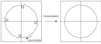
Non-sensitive band and delayed timing before compensation
