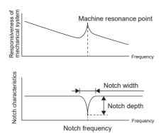
The characteristics of the machine resonance suppression filter change according to notch depth and width selections as follows.
