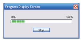
Completing one-touch tuning starts the writing of servo parameters to the servo amplifier. In addition, the following dialog is displayed after completing one-touch tuning. Select whether or not to reflect the tuning result in the project.
