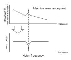
· When machine resonance is small and frequency is high
