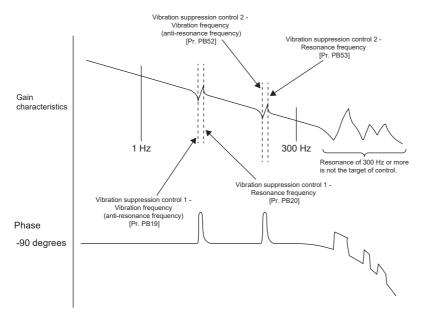
• When vibration can be confirmed using a monitor signal or an external sensor
