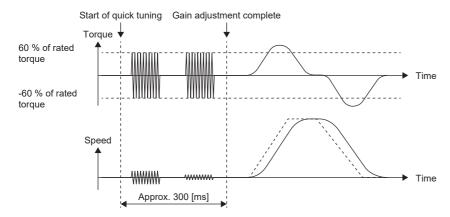
The following servo parameters are adjusted automatically in quick tuning.
