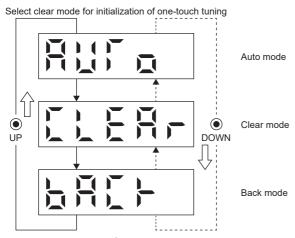
$\downarrow$  To clear the adjustment results of the one-touch tuning, push the "SET" button.
