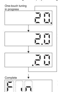
The progress of the one-touch tuning is represented from 0 % to 100 %. The decimal point moves right to left in rotation during the tuning. Pushing the "MODE" button during the tuning switches to the status display.
