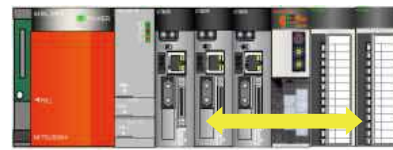
Direct control between CPUs and I/O units
