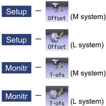
The tool compensation data can be set and displayed tool offset (T-ofs) screen of the setup (Setup) screen.
