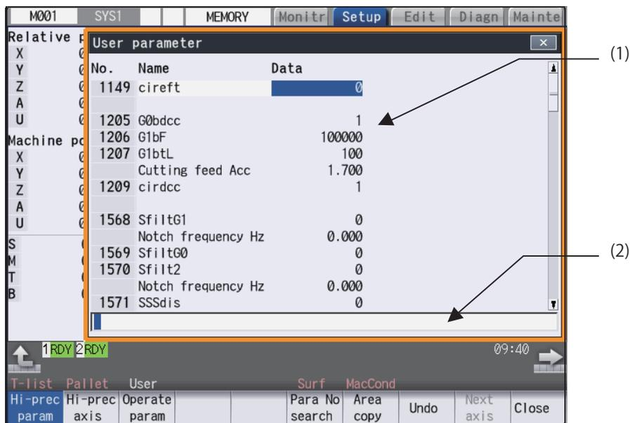
Display example by axis (Switch the fourth axis and after on the menu [Next axis].)
