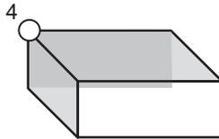
When the workpiece is greatly tilted, confirm the measurement face in the figure on the previous page and set the workpiece zero point so that the stylus bar portion does not contact the workpiece.
