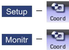
The coordinate system offset and workpiece installation error compensation controlled by the NC can be set and displayed on the monitor (Monitr) screen or the Setup screen.
