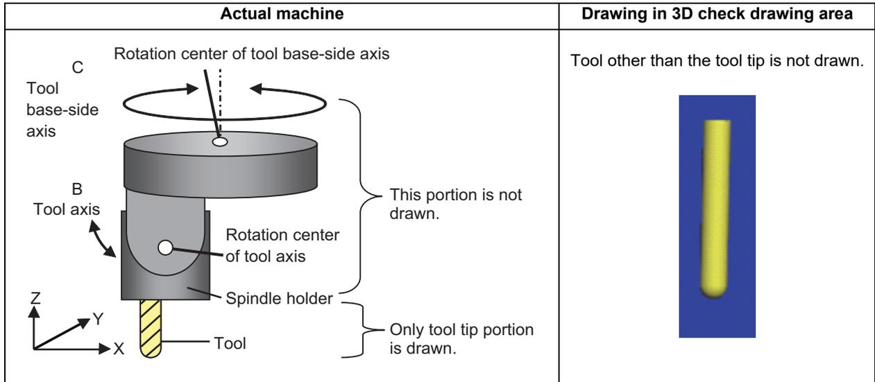
**[Drawing travel command of tool base-side axis]**
