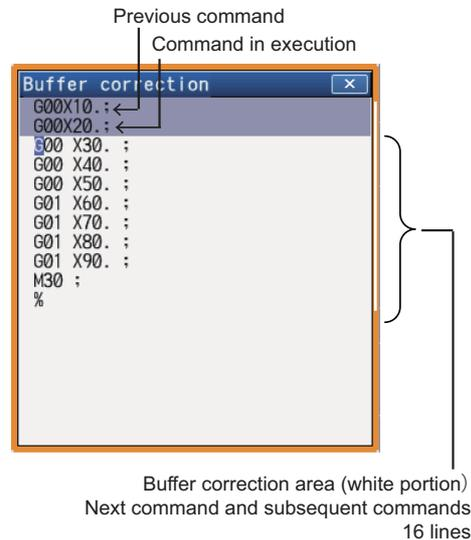
The display changes so that the next command is at the head of the area. The buffer correction area becomes the valid area, and the keys can be input or the cursor moved.
