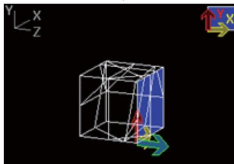
Each time the menu [Graphic Rot] is pressed, the direction of the workpiece graphic is switched in the order of (1) to (4) as shown below:
