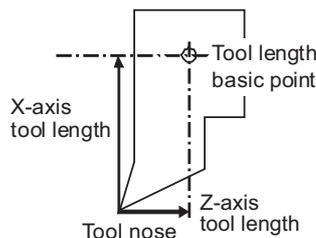
When the tool touches the touch probe while measurement switch is ON, the calculation result is set in the tool data of the compensation No. specified with "Tool No. (Tool length measurement 2)" (PLC device), and the wear data of the compensation No. set in "Wear compensation No. (Tool presetter)" (PLC device) is cleared.
