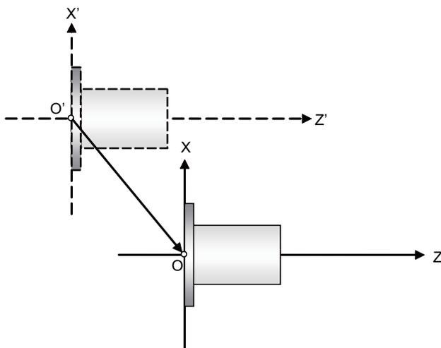
Set the shift value to  $O' - O$  as the shift value of the workpiece coordinate system shift value.
