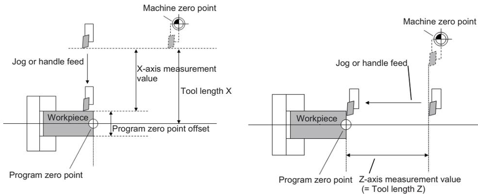
The tool length is automatically calculated by the following formula:
