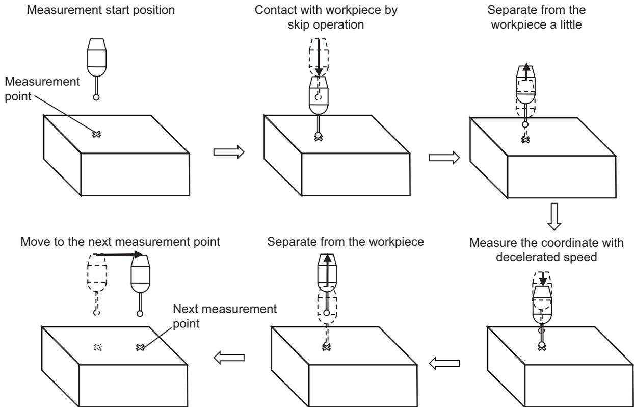
The measurement is started from the position one third away from each side in the direction perpendicular to the measurement face for each measurement point.
