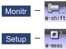
This function allows you to shift the workpiece coordinate system.
