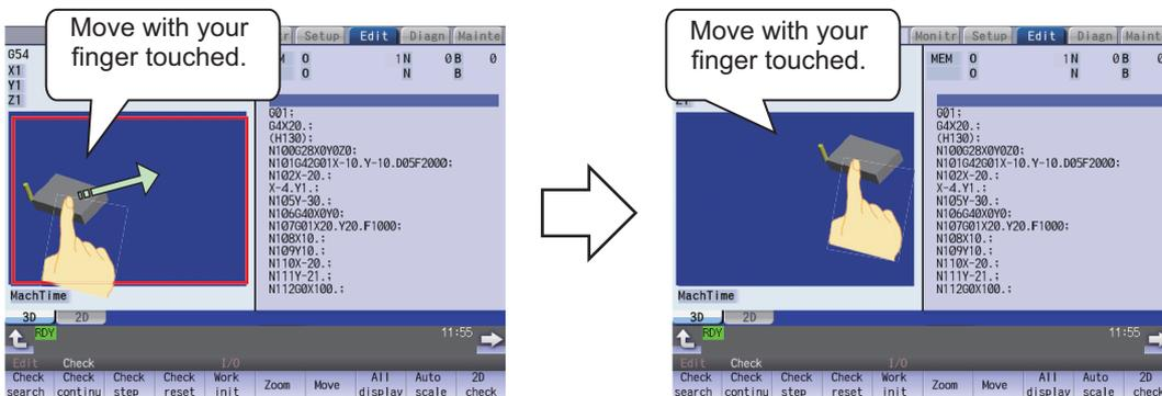
You can rotate a machining shape using a two-finger drag operation (put two of your finger tips on the screen and move them vertically/horizontally without losing contact).
