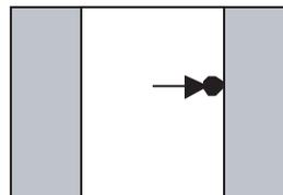
Upon contact, the axis automatically contacts the workpiece again. The skip position displays in the measurement counter point A.
