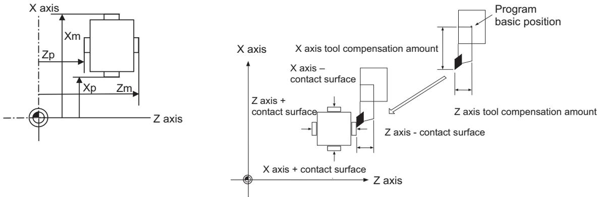
When measured at the main spindle side:
