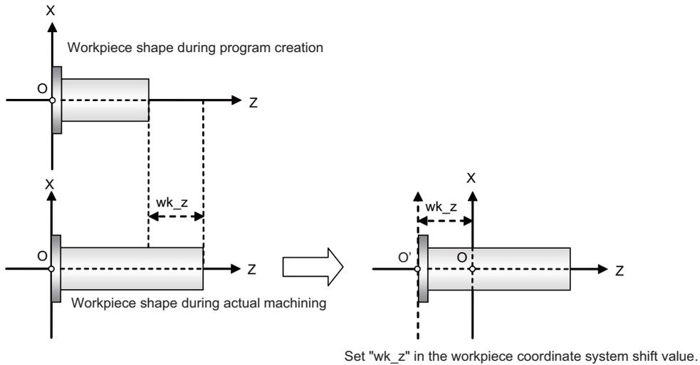
X - Z: Coordinate system established when the program is created
